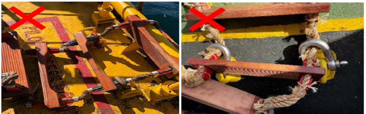
(Examples of non-compliant securing methods using shackles)
